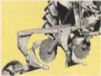
2-bottom, mounted. Simple strong construction and easy to use. There's a choice of spring trip or shear bolt beams, bottoms and accessories.
