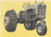
Row crop, single wheel. Power steering is standard—also Rest-O-Ride seat. Front end can be quickly changed to dual wheel or wide adjustable.
