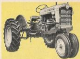
Row crop tricycle. Power steering is standard—also Rest-O-Ride seat. Working weight nearly 6000 pounds, equipped with weights and liquid tire fill. Power adjusted rear wheels.
