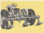
Middlebusters, tool bar. 2 to 5 rows, choice of straight or curved beams, middlebuster or lister bottoms. Truss rods, gauge wheels, extra.
