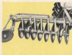
One-way plow. Eight 22 inch discs combined with heavy tubular frame weight to cut up to 6 inches deep. Ideal for muck farming as it mixes surface trash and soil.
