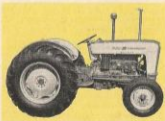
Special utility model. Low cost. No hydraulic system, lights, Rest-O-Ride seat or Proof-Meter. PTO optional. Big bargain for loaders, backhoes or straight drawbar work.
