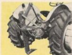
Subsoiler, mounted. Break hard pan up to 18 inches deep. Long wearing chisel reverses. Rugged steel construction. Good clearance.
