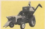
Picker-sheller . Fully mounted—easy to handle. Attaches quickly. 30 bu. tank unloads in 1½ minutes. Cylinder-type sheller.
