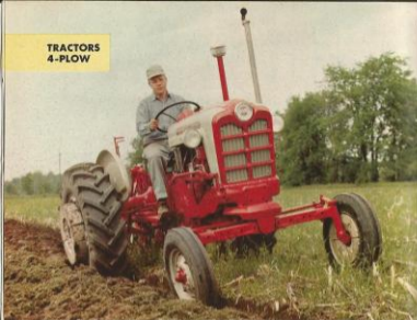
All Purpose. Short 74½ inch wheelbase for short turning. Low 57½ inch hood height for cramped quarters. Easy to get on and off.
