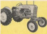
Row crop, wide adjustable. Power steering is standard. 27½ inch crop clearance. Power adjusted rear wheels from 56 to 84 inches.
