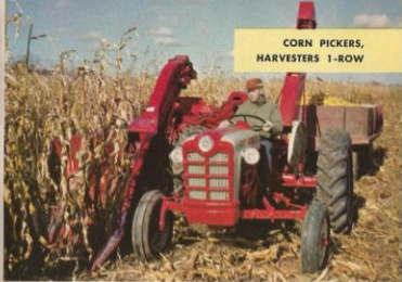
With gathering unit mounted up front, you can stay on the row better
